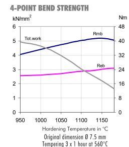
Dimension of test piece Ø 4.7 mm NB: High quality surface Rmb = Ultimate bend strength in kN/mm<sup>2</sup> Reb = Bend yield strength in kN/mm<sup>2</sup> Tot. work = Total work in Nm
