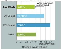
Work material: SCM415 Friction distance: 400m Friction speed: 0.76m/s Load: 67N
