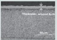
Adherence between the coating layer and steel after 3-time CVD treatment.
